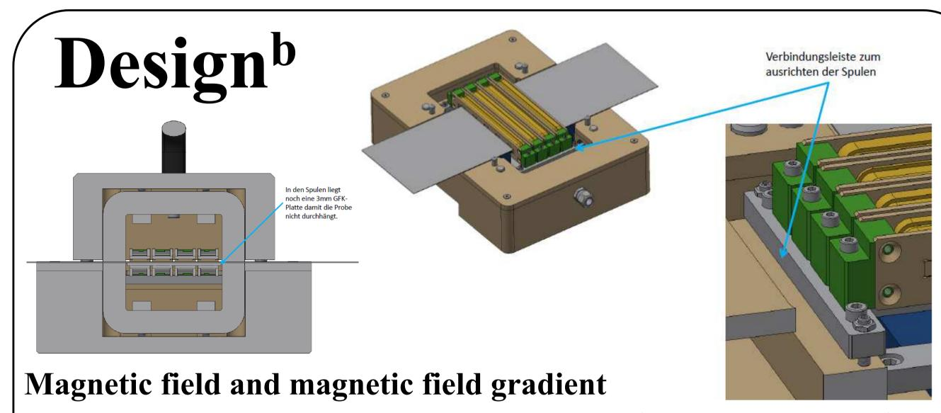
I: 11 turns per coil and per layer. 88 turns in  $1^{st}$  and  $2^{nd}$  layers. 26 turns in  $3^{rd}$  layer (total = 114 turns). Design of two separate coils: coil (Ia) in the  $1^{st}$  and  $2^{nd}$  layer (70 turns) and coil (Ib) in the  $2^{nd}$  layer and  $3^{rd}$  layer (44 turns) to be connected in series.
