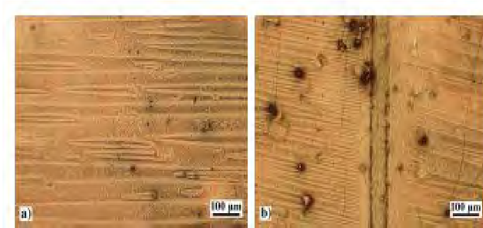
Figure 7: The domain structure of investigated GO steel: (a) without laser scribing and (b) after laser treatment by laser beam in continuous mode with power of 24 W. [30]
