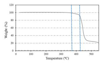
Fig. 7. STA decomposition curve at 20°/min for EP.
