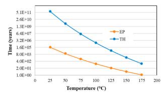
Fig. 8. Life estimation for EP and TH.
