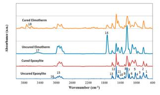
Fig. 11. Normalized absorbance as a function of wavenumber (cm-1) for EP and TH uncured and cured.
