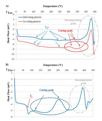
Fig. 2. DSC to measure glass transition temperatures for A) EP and B) TH.
