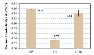
Fig. 10. Thermal conductivity for EP, TH and EPTH.
