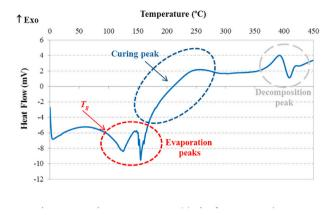
Fig. 6. Heating curve at 20°/min for uncured TH.
