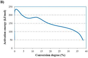
**Fig. 5.** A) Conversion degree curves at different rates for EP and B) Activation energy versus conversion degree for EP.
